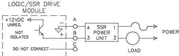
**Logic/SSR Drive:** Can drive multiple SSR Power Units.
