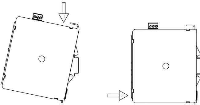
**Figure 1 - Attach ICM8 To DIN Rail**
