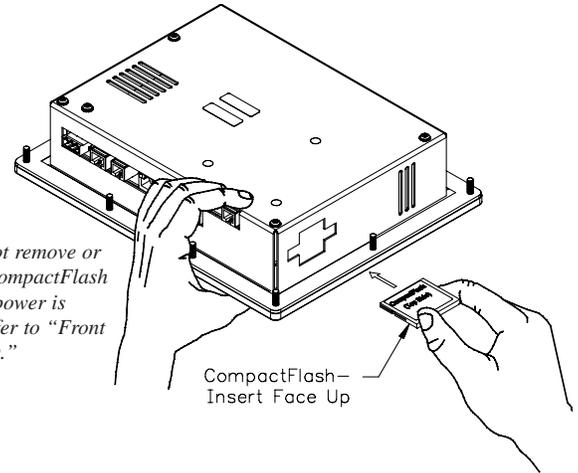
Information stored on a CompactFlash card by a G308 can be read by a card reader attached to a PC. This information is stored in IBM (Windows®) PC compatible FAT16 file format.
